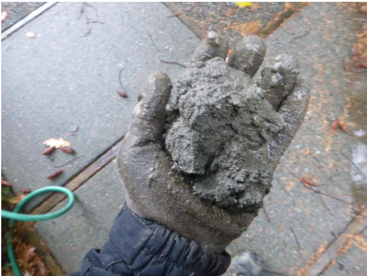
Plate 1. Cuttings from about 3 feet below the surface in HB-2. Wet, gray, medium SAND with trace silt.
